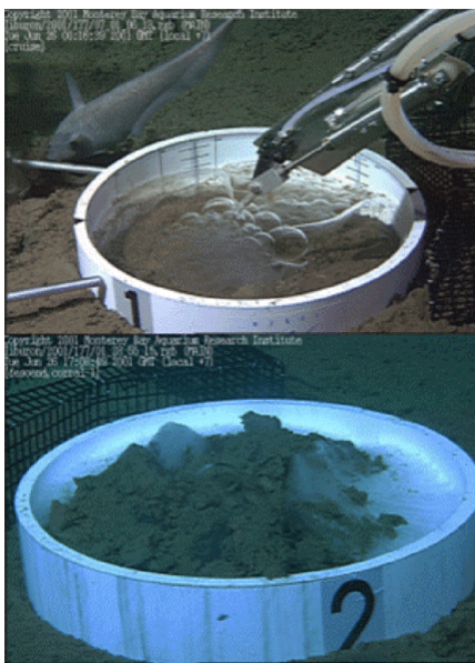
Figure 6.10. Liquid CO 2 released at 3600 metres initially forms a liquid CO 2 pool on the sea floor in a small deep ocean experiment (b, upper picture). In time, released liquid CO 2 reacts with sea water to form a solid CO 2 hydrate in a similar pool (b, lower picture).
